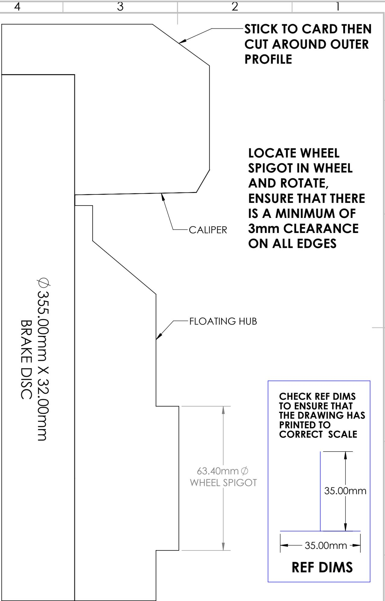
CHECK REF DIMS TO ENSURE THAT THE DRAWING HAS PRINTED TO CORRECT SCALE
