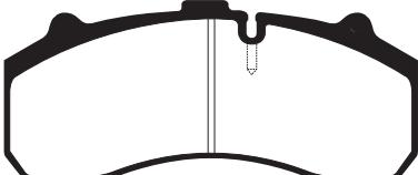
Pad has drilled wear receptor hole in line
