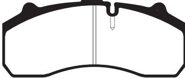
Pad has drilled wear receptor hole in line with cutout
