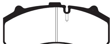
Pad has drilled wear receptor hole in line with cutout
