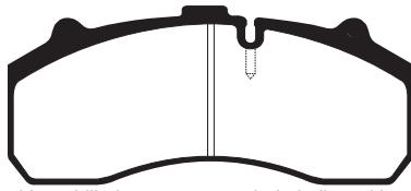
Pad has drilled wear receptor hole in line with cutout
