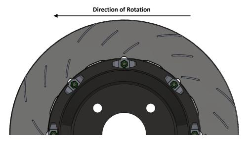
**WARNING!** DO NOT REMOVE THE BRAKE DISC FROM THE BELL. For composite discs, the bells are also subject to wear, therefore replacement of a worn floating disc involves complete replacement of the assembly and not only the disc.
