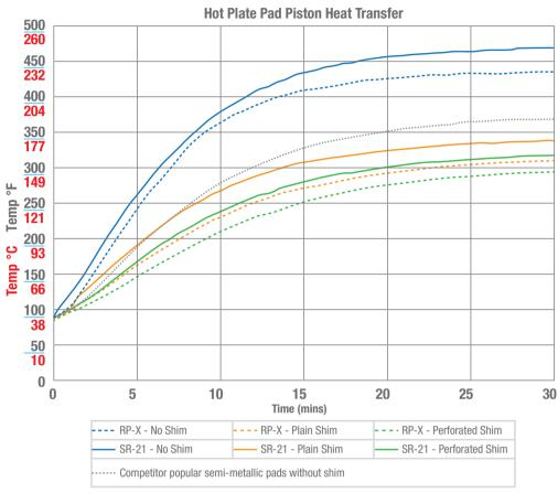
These tests were conducted to compare the heat transferred with plain shims or perforated shims and EBC race materials were used. However, the physics remains sound and any semi-metallic pad should benefit from shim heat insulation.
