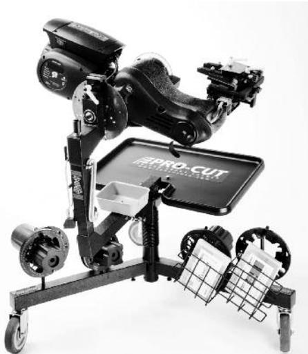
Pro-Cut's PFM 9.2DRO on-car brake lathe
